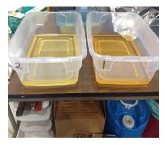
Place parts in initial bath for 3-5 minutes to remove wax from fine features.
