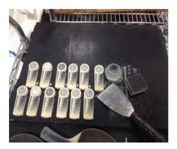
3. Keep Angle of putty knife below 20 degrees to avoid scraping platform.
