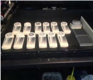
Note: Leaving parts in Freezer for extended period of time can cause parts to distort.
