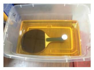
4. If parts have small crevices which retain bits of wax (e.g. meshes, small internal geometries) a heated ultrasonic cleaner at 65-70°C can be used in place of bins. Ultrasonic cleaners help vibrate the wax in the small crevices.
